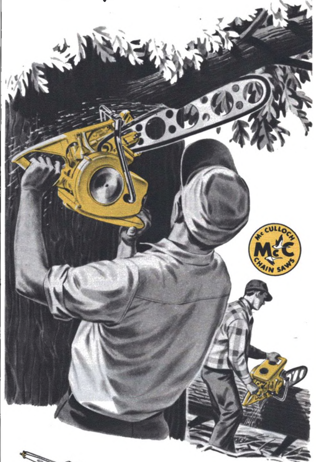
This 5-horsepower McCulloch chain saw is available with blades up to 5 feet long.
